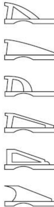
Rear bumper must be capped, with no sharp edges, and bent forward on the ends at a 90°degree angle.
